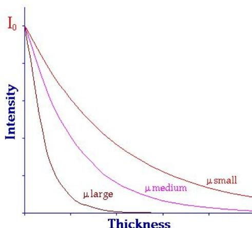
A material's **linear attenuation coefficient ( $\mu$ )** is a measure of how easily a beam of X-rays (for example) can pass through it, and **describes the rate of energy loss per unit thickness**. This value **depends on the density** of the material, as a **higher density material will absorb more energy as there are more atoms for the photons to encounter**.
