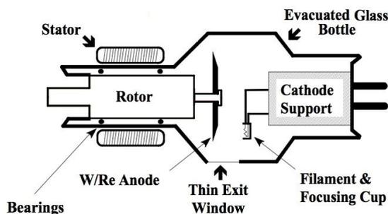
To prevent overheating, the **metal target/anode is also rotated at high speeds** (around 3000 revolutions per minute) so that the electron beam heats different areas of the target. The metal
