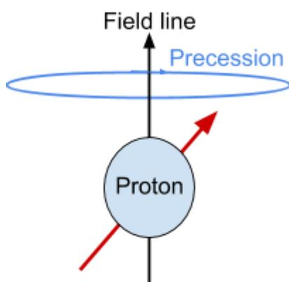
Radio frequency coils are used to produce **pulses of radio waves (radio frequency (RF) pulses)** at different frequencies, which causes protons with the same precession frequency as the
