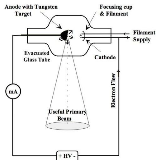
The **maximum X-ray photon energy** produced by the above method is equal to the **product of the charge on the electron**
