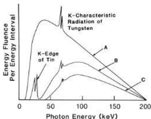
The image on the left shows the effect of 3 different types of filter on the intensity of radiation:
