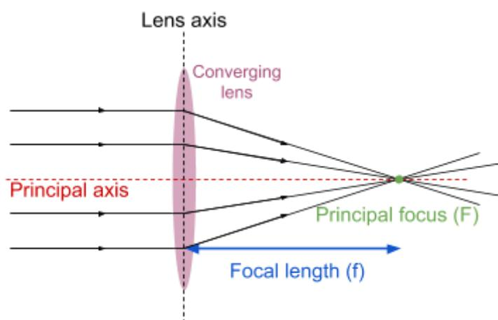
You can use **ray diagrams** in order to map where an image will appear after passing through a lens. To draw a ray diagram:
